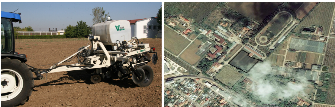
Fig. 1. System for mapping the electro-conductivity of the Veris 3150 soil with the electro-conductivity (center) and ph (rear) sensors
